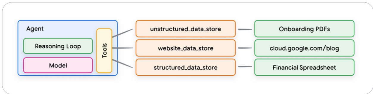
Figure 12. 1-to-many relationship between agents and data stores, which can represent various types of pre-indexed data
